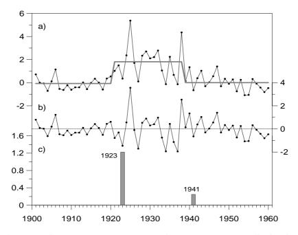
**Fig. 1.** a) A synthetic time series consisting of three segments of normally distributed random numbers with the following mean values and variances: 1) 0, 0.5, 2) 2, 4, and 3) 0, 0.5. Gray line is the stepwise trend showing regime shifts in the mean detected by the sequential method; b) the same time series after removing the stepwise trend; and c) RSSI showing regime shifts in the variance.
