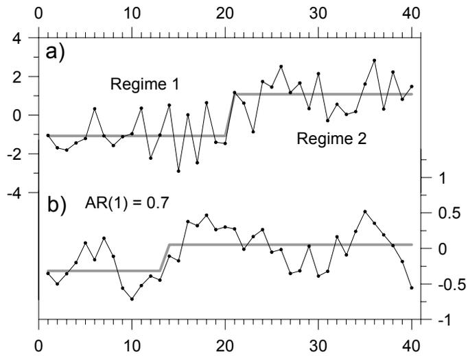
**Fig. 1.** Realizations of a) white noise process ( $\sigma^2 = 1$ ) with a shift in the mean at  $t = 21$  from  $\mu_1 = -1$  to  $\mu_2 = 1$ , and b) red noise process with  $\rho = 0.7$ . The shift at  $t = 14$  in the latter case would be statistically significant at the 0.05 level, if the data points were independent.
